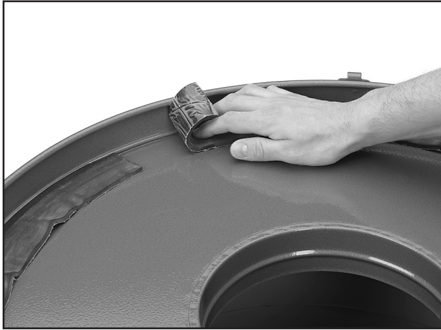
Figure 34. Applying dust collection drum lid gasket.
